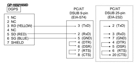
Figure 10-17 Connection of GP-1650D/GP-1650 to PC
